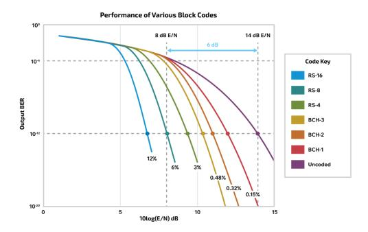
We can see from the graph that implementing RS (255,239) FEC code will improve the BER from  $10^{-4}$  to  $10^{-12}$  at an E/N ratio of 8 dB. This is a 6 dB E/N improvement from the uncoded case, where E/N has to be 14 dB to achieve the BER  $10^{-12}$  performance.
